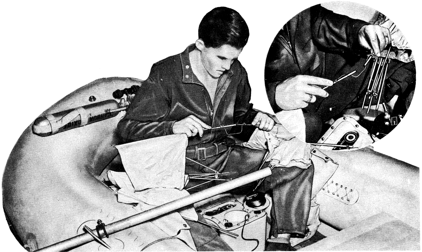
Figure 17—Kite M-357-A, Assembly Operation
